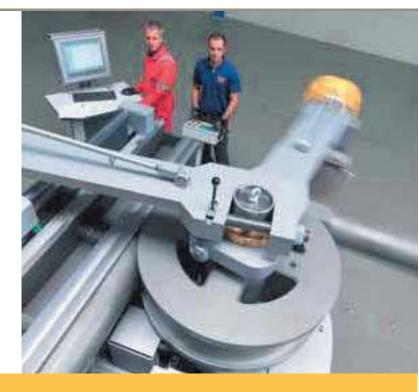
The Parflange F37 program is operation-friendly and environmentally friendly technology. Production times are reduced by more than half when compared to conventional welding.
